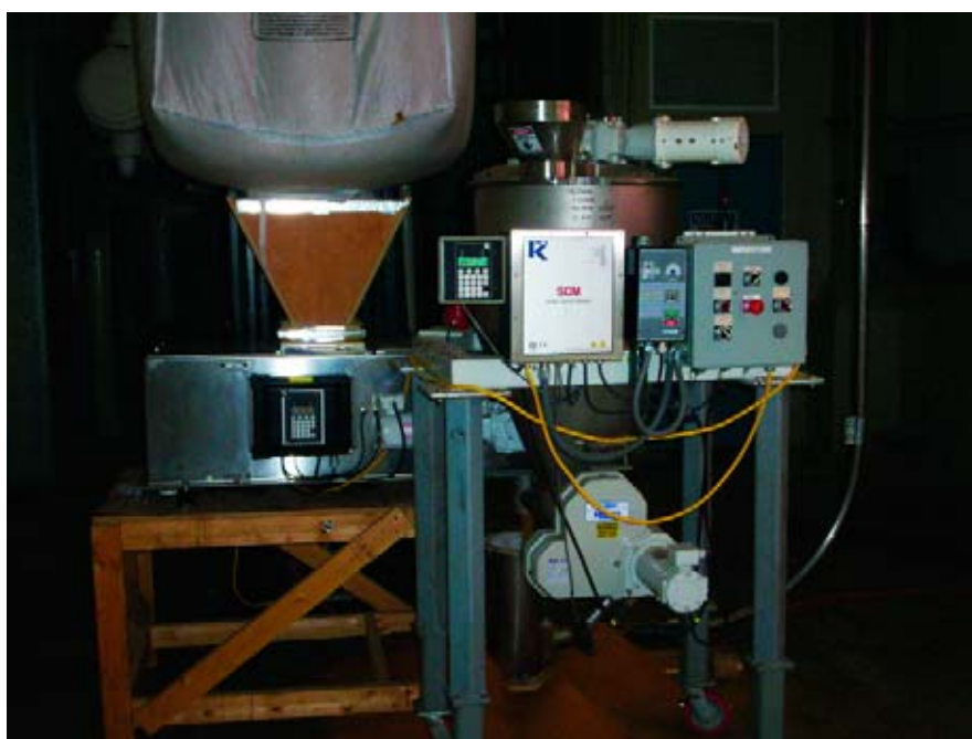
The weighbelt feeder (left) and portable LIW feeder (right) each meter cornmeal into the vacuum conveying system.
